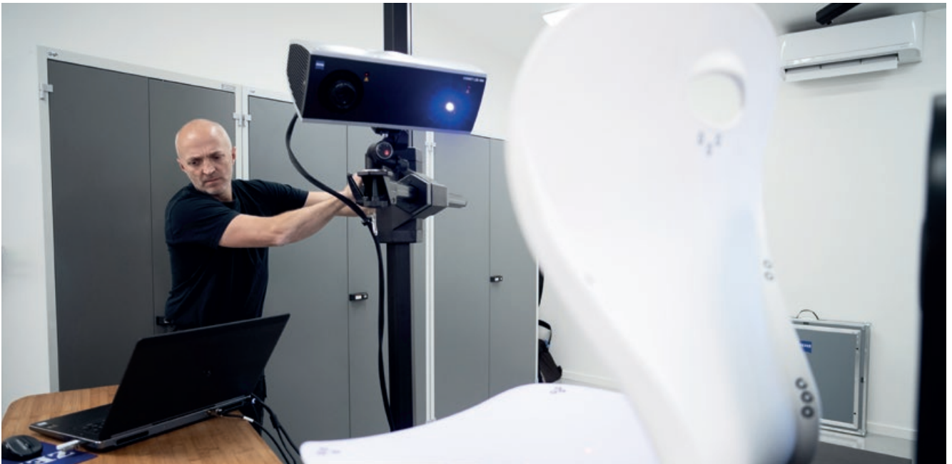
Frank Fynbo examines the seat shell of a chair with a 3D scan of ZEISS COMET. The plastic part was produced using 3D printing.
