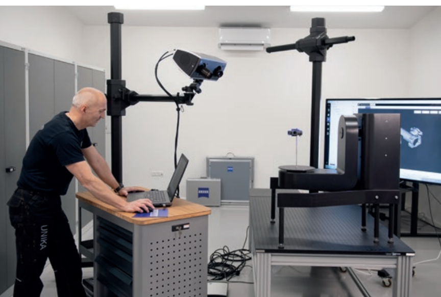
Frank Fynbo at ZEISS COMET. The setup of the 3D scanner and the measurement only take a few minutes.
