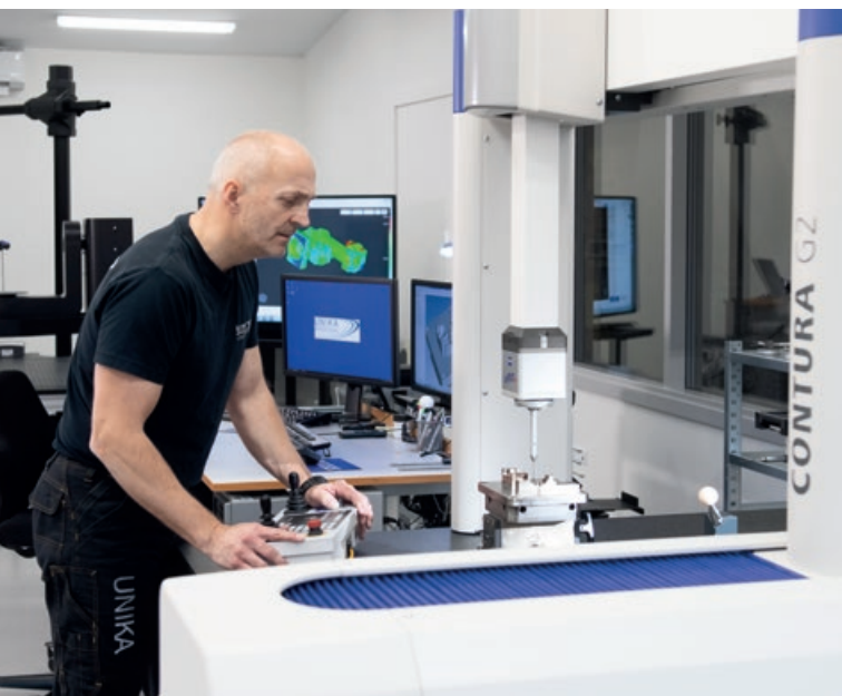
Precise injection molding tools are required for precise plastic parts. A CONTURA coordinate measuring machine from ZEISS ensures their quality at Unika.
