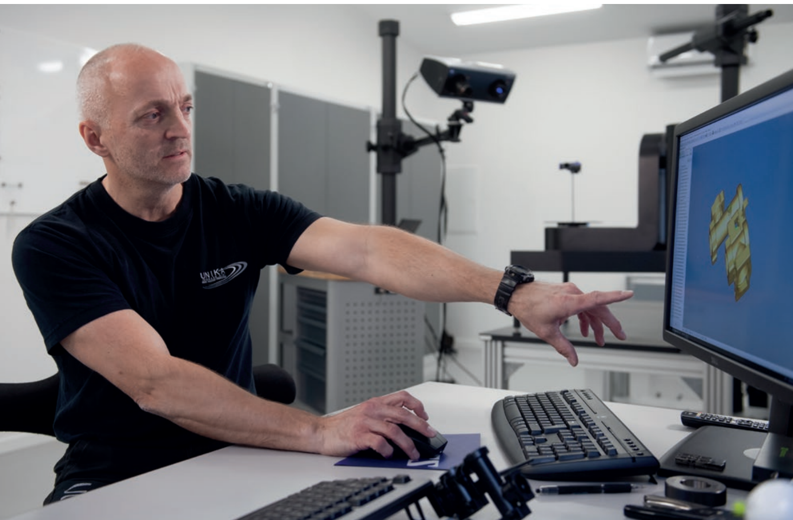
Frank Fynbo examines the casing of a water pump. Whether all measurements are correct, he can decide however only after the examination with the 3D sensor.
