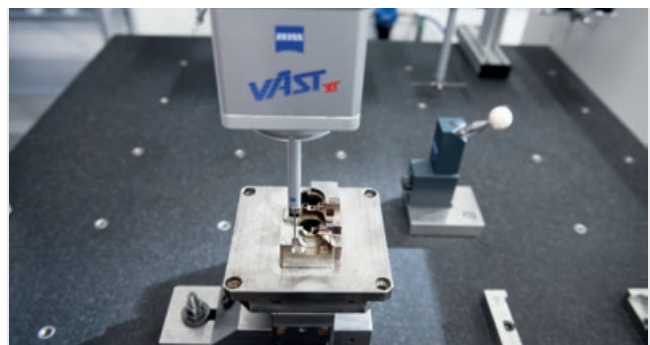
Precise injection molding tools are required for precise plastic parts. A CONTURA coordinate measuring machine from ZEISS ensures their quality at Unika.
