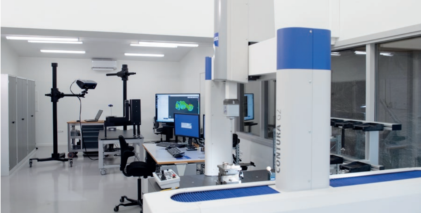
Unika relies on ZEISS precision: With COMET and CONTURA, injection molding tools and parts can be measured with high precision.
