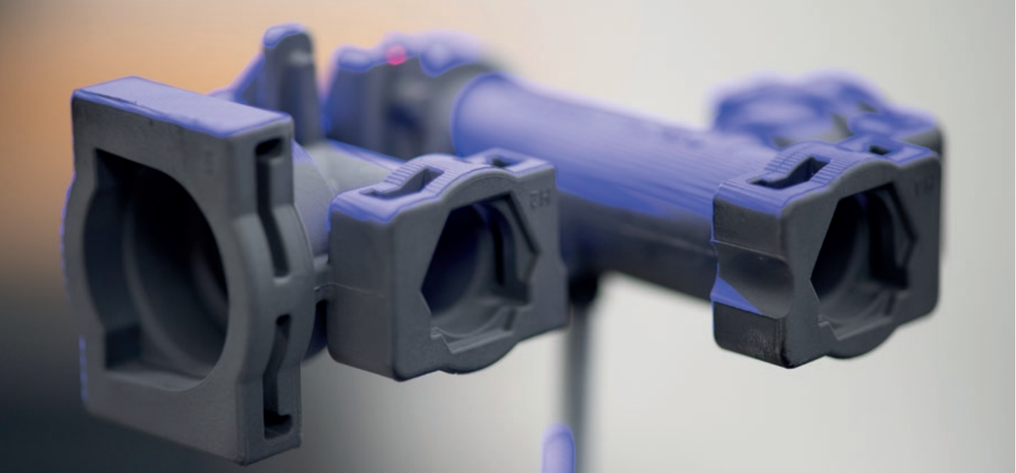
The plastic housing of a water pump glows blue under the laser light of the ZEISS COMET 3D scanner.
