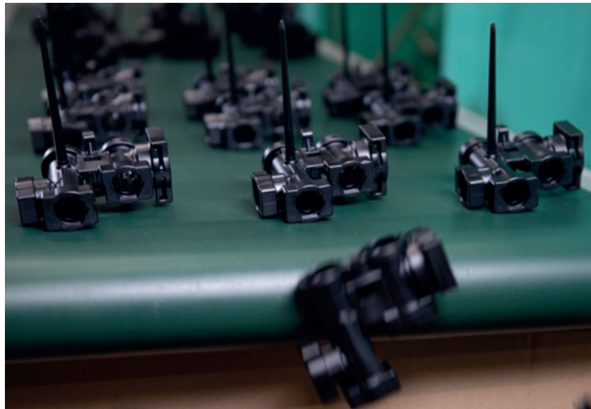
After leaving the injection molding machine, the plastic parts cool down on a conveyor belt. The finished injection molded parts are collected in a box and brought to the customer.
